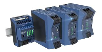
The RACPRO1-T240, -T480, and -T960 power supplies deliver 240W, 480W, and 960W, respectively. All members of the family support a universal, threephase AC input voltage range of 3x320VAC to 3x576VAC. The family also supports a universal DC input voltage range from 430VDC to 850VDC, allowing the parts to support renewable energy and micrgrid applications.
