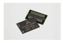
A new monolithic high-speed, low-voltage CMOS double data rate 3 synchronous DRAM (DDR3L SDRAM) with an 8-Gb density in the 78-ball, 9-mm by 13.2-mm, lead (Pb)-free FBGA package. Delivering increased power efficiency for high-end computer and storage systems, the 1G x 8 AS4C1G8MD3L offers a double data rate architecture for extremely fast transfer rates of up to 1600 Mbps/pin and clock rates of 800 MHz.
