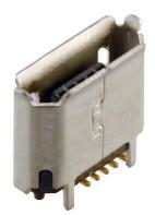
Kycon has expanded their USB series, adding a vertical mount micro USB B-type connector to increase versatility in their line. The vertical mounting option offers a design solution where board space is a concern. The KMMVX-SMT series comes standard with gold flash plating and tape-and-reel packaging with a cap for pick and place. 50u gold plating is available upon request.
