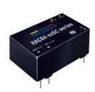
The converters are in an encapsulated PCB-mount package style with 3.75kVAC isolation and very low stand-by power consumption. The converters have SC protected single as well as dual outputs and meet EN55022 class B without any external components. The module is a pin-compatible redesign of the RAC04-SA/SB series but with better specs and lower price. Uses include board-level power supplies, home automation, instrumentation systems, and standby applications.
