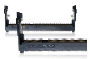
With these two new series, Yamaichi is expanding its large family of production use and Test & Burn-in sockets. The two new sockets are for production usage. The CN111S socket was developed especially for modules that meet the DDR2 (Double Data Rate) standard in the SO-DIMM version (Small Outline Dual Inline Memory Module). It is a 200 pin 1.8V version with an installation height of 5.2 mm. The contacts are gold-plated as standard.
