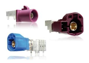
FAKRA connectors (FAKRA is derived from German for Automobile Working Group, Fachkreis Autombil) are coaxial high-frequency connectors that meet the requirements of DIN20860 and USCAR 17 & 18. Their application lies in the transmission of a variety of signals, such as shortwave, mobile telephony, GPS, or telematics signals. Thanks to standardization, each application is assigned a specific colour and
