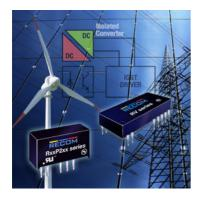
The modules are available with input voltages of 5VDC, 12VDC & 24VDC and offer up to 6.4kVDC/1sec isolation. The converters operate reliably at temperatures between -40 °C and +90 °C without de-rating and with an efficiency of up to 85%.
