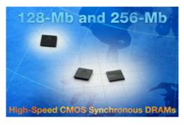
The AS4C8M16S-7BCN and AS4C16M16S-7BCN is optimized for medical, industrial, automotive and telecom applications requiring high memory bandwidth. They are particularly well-suited to high-performance PC applications. These components operate from a single +3.3-V (± 0.3 V) power supply and are lead (Pb) and halogen-free.
