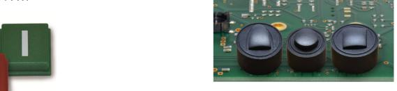
Another addition to our product range is legends on Varimec caps. Varimec caps are made of nylon as standard. Legends can be printed on the nylon, but the lifetime is less than in case of other materials MEC provides. To overcome this, legends can be printed on Varimec caps made in polycarbonate material. Due to the low temperature range of the material the cap has to be mounted after the soldering process. Varimec caps in polycarbonate with legends are custom products.
