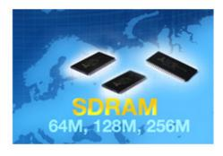
Packaged in a 54-pin, 400-mil plastic TSOP II, the new SDRs offer a fast access time from clock down to 4.5 ns at a 5-ns clock cycle and clock rates from 143 MHz to 200 MHz.
